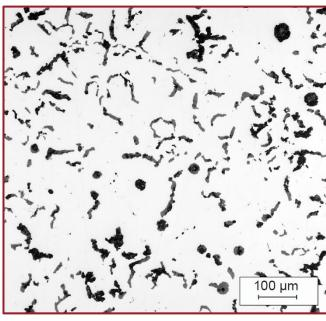
Figure 1: CGI microstructure containing 10% nodularity
