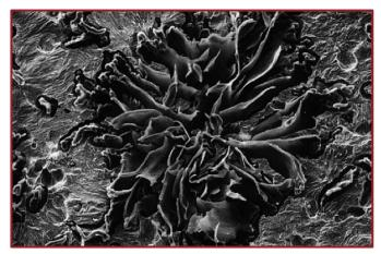
Figure 2: Individual flake patches form when magnesium treatment is insufficient
