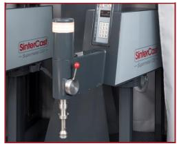
Re-engineered SAM with improved Thermocouple Holder
