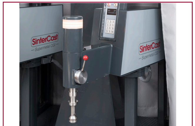
Re-engineered SAM with improved Thermocouple Holder
