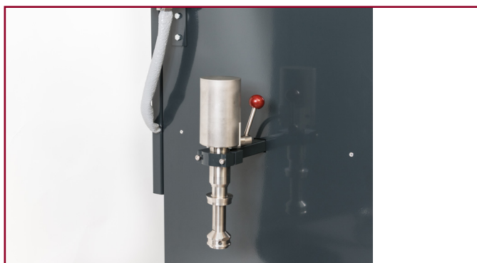
Re-engineered SAM with improved Thermocouple Holder
