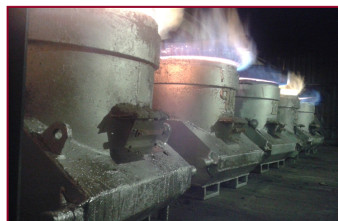
RFID Ladle Tags affixed to each ladle
