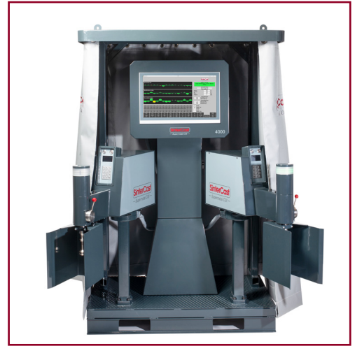
Fully Automated System 4000 with two Sampling Modules
