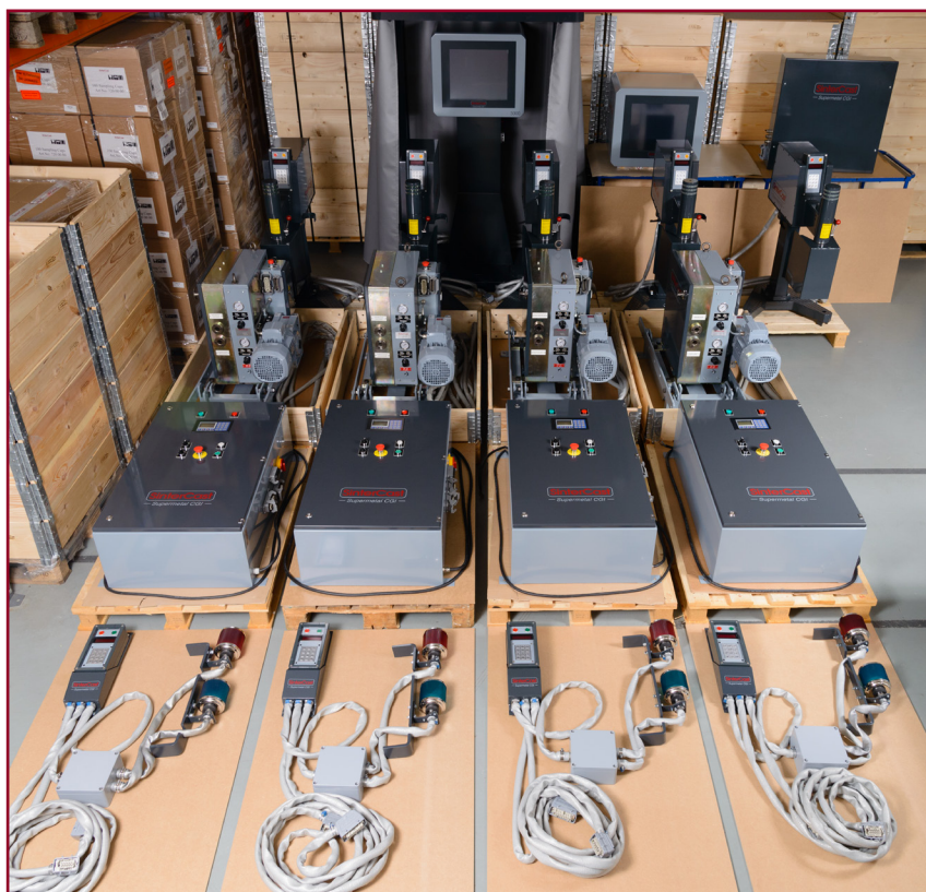
SinterCast's first-ever System 3000 Plus installation was announced on 29 October 2012. Configured with four wirefeeders and five Sampling Modules, the System 3000 Plus will be commissioned at the Tupy Saltillo foundry in Mexico during March-April 2013 and is specified to support the production of 15 ladles per hour, with more than nine hours of series production every day.
