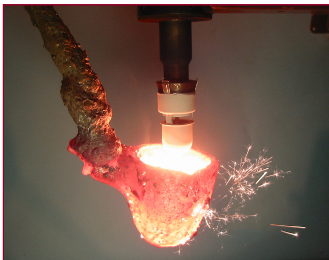
SinterCast's unique immersion sampling
