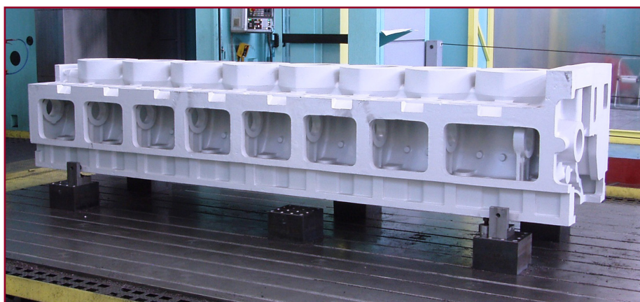
SinterCast's largest casting during 2013 was a 9 tonne engine entablature for Allen Diesels of the UK. With CGI entablatures and heads, the Allen Series 4000 engines provide power outputs from 1,800 to 5,050 kW in power generation applications around the world. (Courtesy Allen Diesels)
