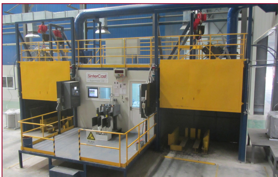
System 3000 Plus base treatment and correction stations at the Zhongding Power foundry, China (Courtesy Zhongding)
