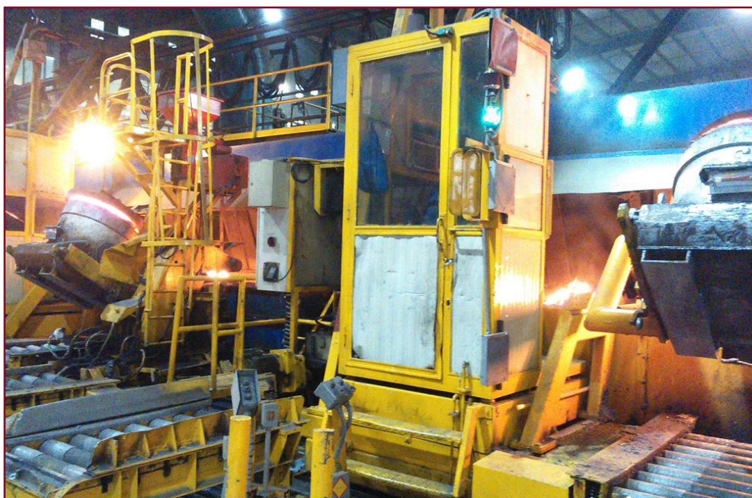
System 3000 Plus: parallel pouring of Ford 2.7 litre V6 petrol engine cylinder blocks at the Tupy Saltillo foundry in Mexico (Courtesy Tupy)
