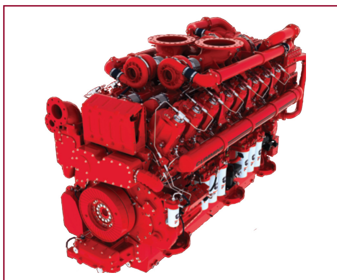
Introduced in 2015, the 95 litre, 16-cylinder, 4,400 horsepower Cummins QSK 95 industrial power engine uses SinterCast-CGI cylinder heads (Courtesy Cummins)
