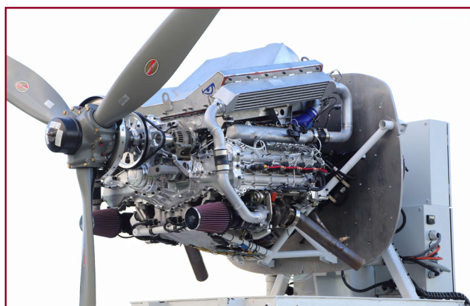
During 2015, Engineered Propulsion Systems began Federal Aviation Authority approval of the first aviation engine with a CGI cylinder block (Courtesy EPS, Inc.)
