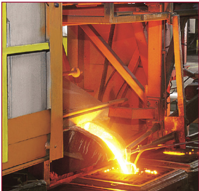
Pouring CGI at the Tupy foundry in Brazil (Courtesy Tupy)
