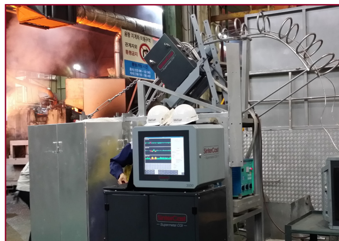
Doosan Infracore, Korea, installed a second Mini-System 3000 during 2015 for the production of a new 27 litre severe-duty engine (Courtesy Doosan Infracore)
