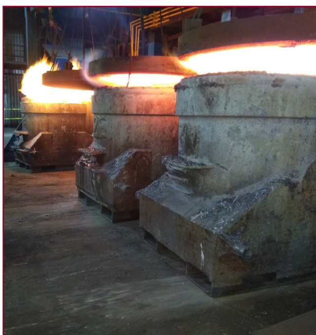
Ladle Tracker ladles on pre-heat at the Tupy foundry in Saltillo, Mexico
