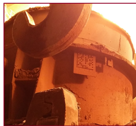
RFID Tags or 2D optical matrix plates (shown) can be used to identify ladles
