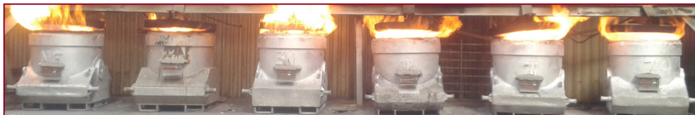
RFID Tags or 2D optical matrix plates enable ladles to be traced throughout the process, linking each mould to the liquid metal history
