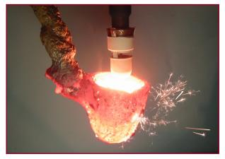
SinterCast Immersion Sampling
