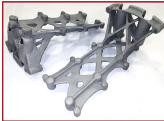
d) Ladderframe castings after shotblasting
