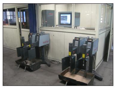
Figure 5: SinterCast System 3000 Plus – SAMs and OCM
