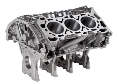
Figure 3: Ford's state-of-the-art 'Nano' V6 petrol engine is based on a CGI cylinder block with parent bore cylinders, fracture split main bearings, and 2.5 mm minimum wall thickness. The entire load path is comprised of CGI
