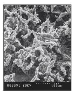
*Figure 2: Deep-etch SEM photo of* CGI microstructure
