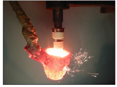
Figure 4: The SinterCast Sampling Cup provides more consistent sampling conditions and better resolution than conventional sand cups
