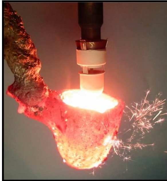
Figure 7: The SinterCast Sampling Cup provides more consistent sampling conditions and better resolution than conventional sand cups.
