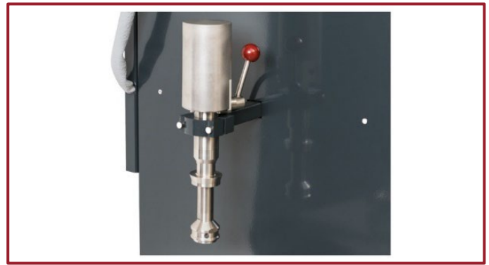
Figure 3: Re-engineered SAM with improved Thermocouple Pair Holder
