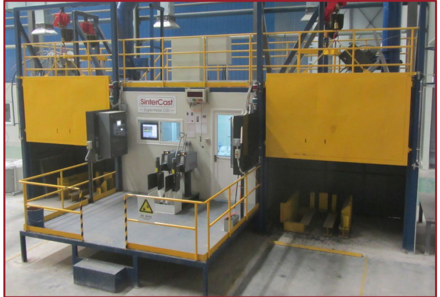
Figure 1: System 4000 Plus base treatment and correction stations
