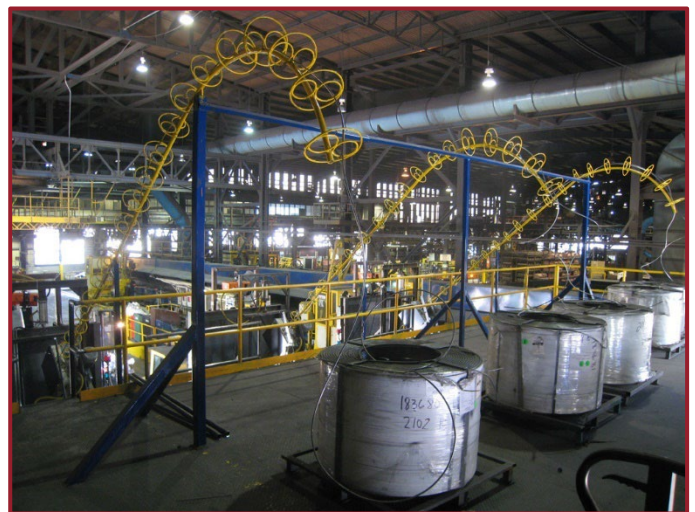
Figure 6: Multiple wirefeeders for base treatment and correction
