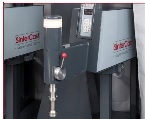
Re-engineered SAM with improved Thermocouple Holder
