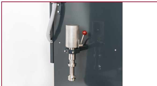
Re-engineered SAM with improved Thermocouple Holder
