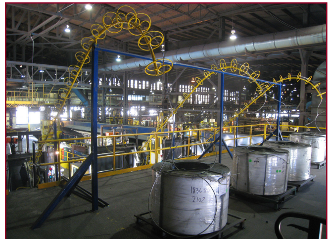
Figure 4: Multiple wirefeeders for base treatment and correction
