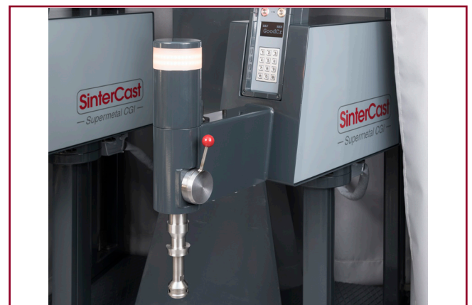
Figure 3: Re-engineered SAM with improved Thermocouple Holder
