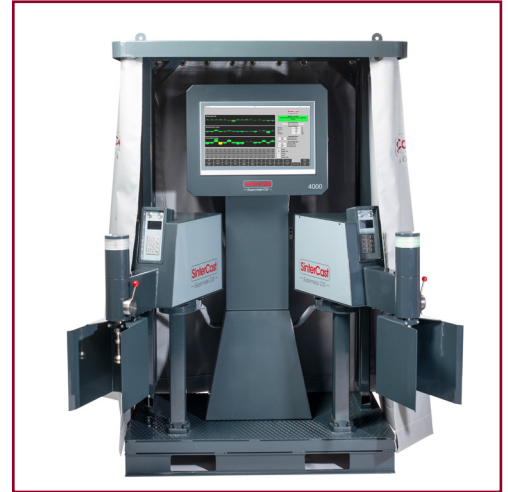
Figure 1: Fully Automated System 4000 with two Sampling Modules
