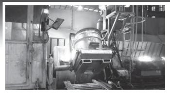
Figure 10: Ladle Tracker<sup>TM</sup> at semi-automatic pouring line.
