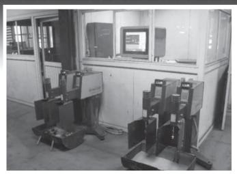
Figure 5: SinterCast System 3000 Plus - SAMs and OCM.
