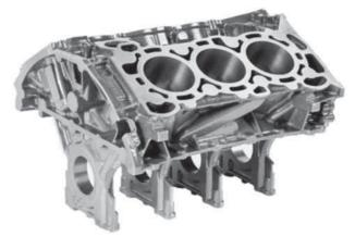
Figure 3: Ford's state-of-the-art 'Nano' V6 petrol engine is based on a CGI cylinder block with parent bore cylinders, fracture split main bearings, and 2.5 mm minimum wall thickness. The entire load path is comprised of CGI.
