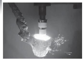
Figure 4: The SinterCast Sampling Cup provides more consistent sampling conditions and better resolution than conventional sand cups.
