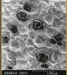
Top to Bottom: gray iron, CGI and ductile iron microstructures. According to SinterCast, the elongated graphite flakes in gray iron provide good heat transfer but reduce strength. The individual spheres in ductile iron provide strength but impair thermal conductivity, the company said. The coral-like compacted graphite microstructure provides strength and heat transfer, SinterCast said.
