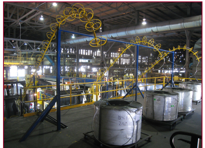
Figure 4: Multiple wirefeeders for base treatment and correction
