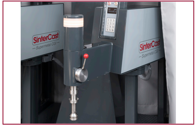
Figure 3: Re-engineered SAM with improved Thermocouple Holder
