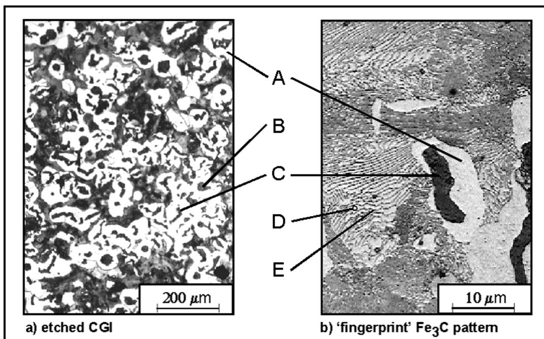
Figure 7: The pearlite phase is an ordered layering of ferrite and Fe<sub>3</sub>C plates (A: free ferrite, B: pearlite, C: graphite, D: ferrite band, E: Fe<sub>3</sub>C plate)
