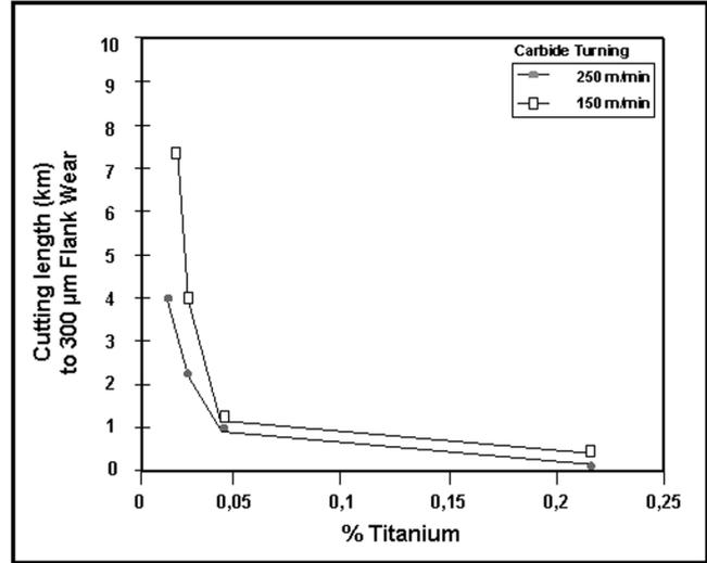
Figure 15: The addition of titanium dramatically reduces the tool life of compacted graphite iron during carbide turning
