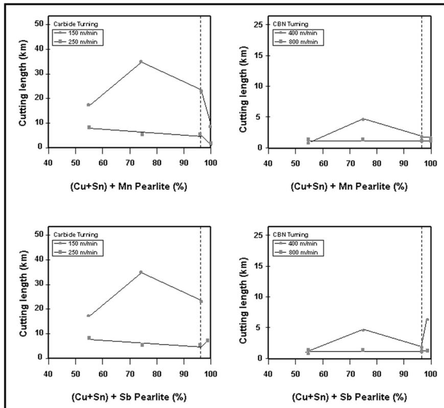
Figure 10: The effect of an incremental increase from 97.5% pearlite (Cu+Sn) to 99% (Sb-CGI) and 100% (Mn-CGI) pearlite on tool life during carbide and CBN turning
