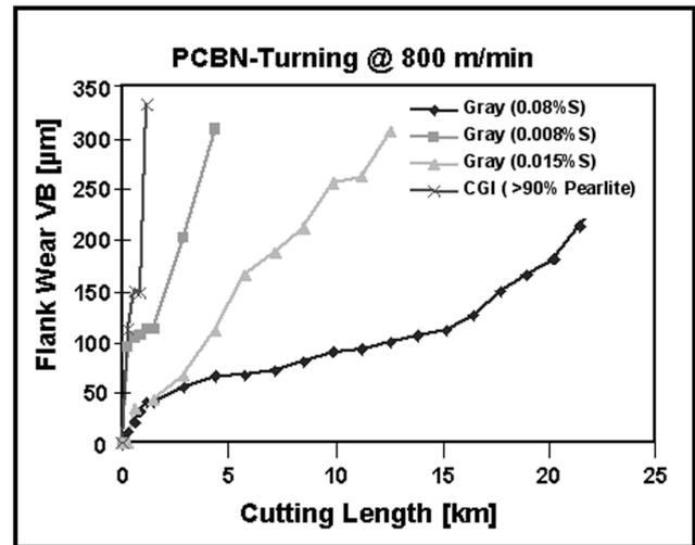
Figure 13: The machinability of grey cast iron gradually decreases as the sulphur content is reduced from, normal grey iron levels (0.08%S) to normal CGI levels (0.008%S)
