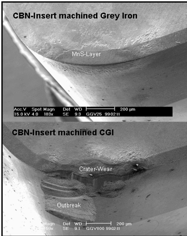
Figure 12: Protective MnS layers form on the cutting edge of PCBN inserts when cutting grey iron at high speeds. In contrast, inserts used for CGI exhibit abrasive wear
