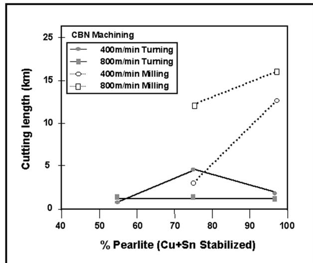
*Figure 9: The effect of pearlitic content on tool life during CBN milling and turning. The pearlite was stabilized by additions of copper and tin*
