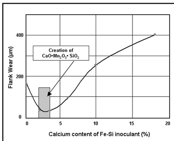
Figure 16: A grey iron inoculant containing 2-3% calcium optimizes the ability to form a protective layer on a TiC coated insert [7]
