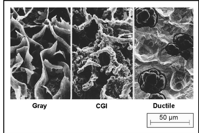
Figure 1: Grey iron, compacted graphite iron and ductile iron are differentiated by the shape of the graphite particles
