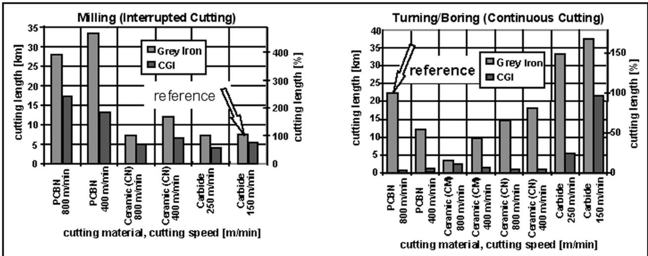
Figure 3: Comparative tool life for different tool materials in interrupted (milling) and continuous (turning/boring) cutting of 70-80% pearlitic CGI and grey iron
