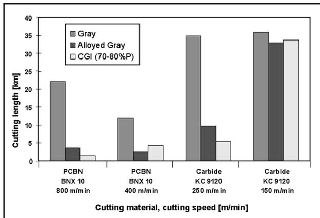
Figure 5: Tool life for conventional grey iron, alloyed grey iron, and 70-80% pearlitic CGI for PCBN and carbide turning
