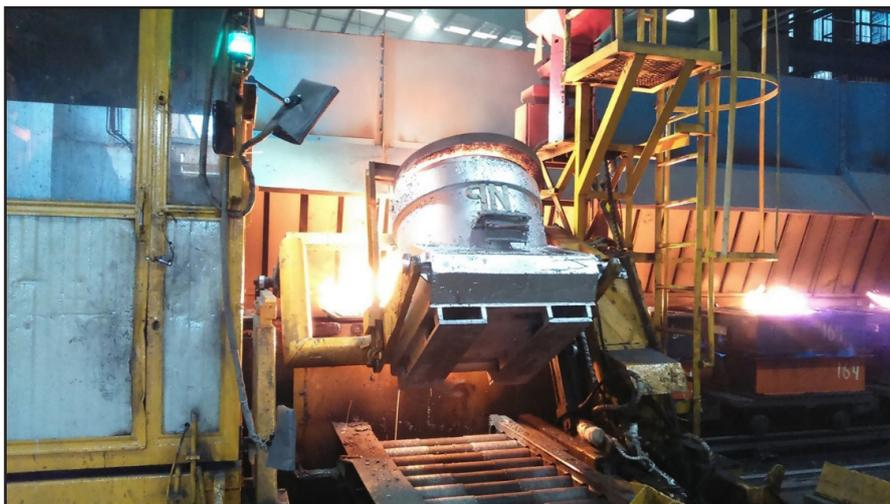
*Figure 10: Ladle Tracker™ at semi-automatic pouring line*
