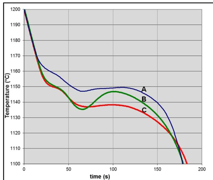
Figure 4: A The differences in the nucleation and growth behaviour of graphite flakes, worms and nodules provide distinct differences in the cooling curves for grey iron (A), CGI (B) and ductile iron (C).
