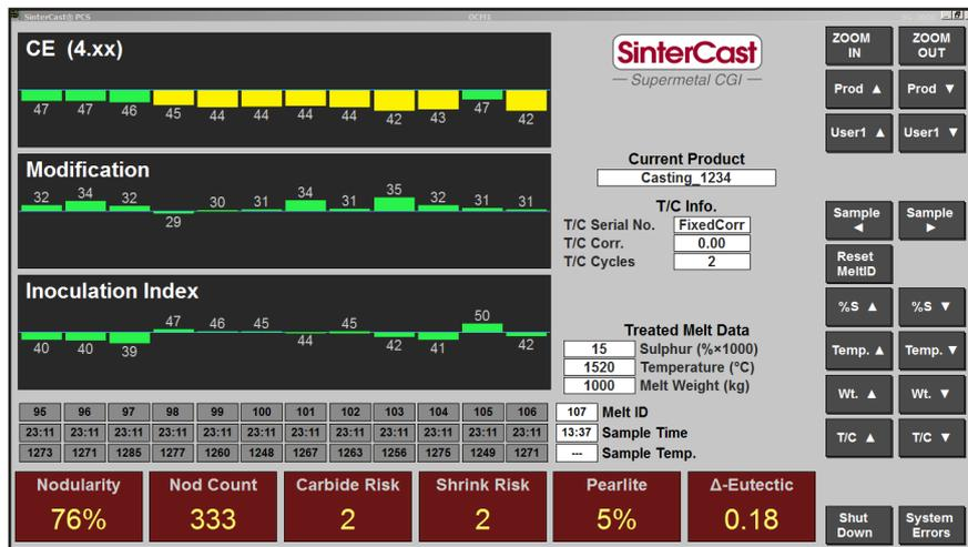
Figure 7: The primary output values of the thermal analysis are the Carbon Equivalent, the Modification index and the Inoculation index. Together, these parameters define the size and location of the calibration window for each individual component and can be used to predict the microstructure and the risk for casting defects.
