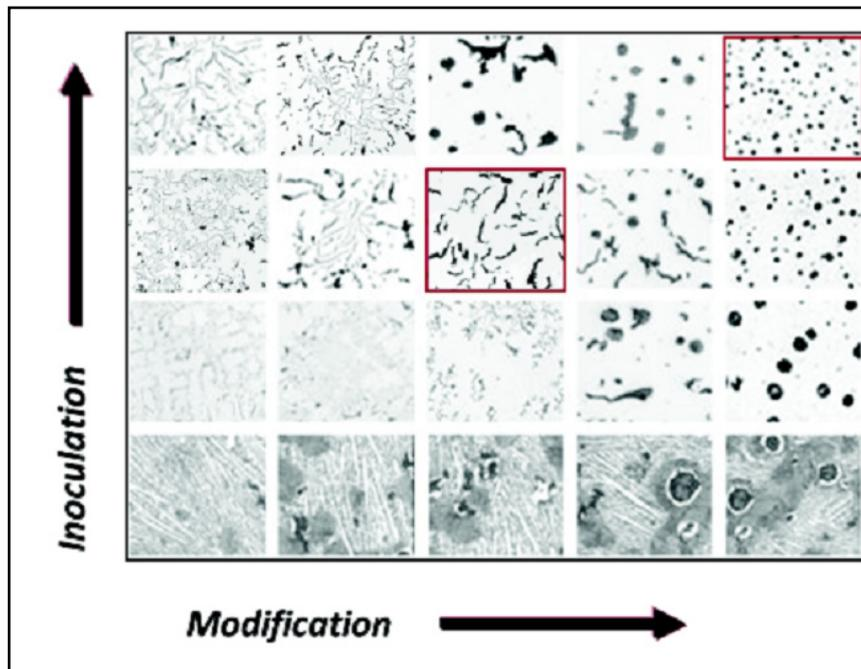
Figure 1: The microstructure chessboard provides a platform for defining the control limits of the stable windows for CGI and ductile iron production.
