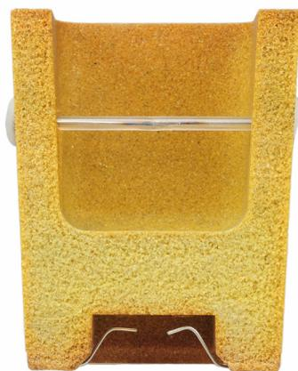
(a) Conventional thermal analysis sand cup with open surface and variable wall thicknesses.
