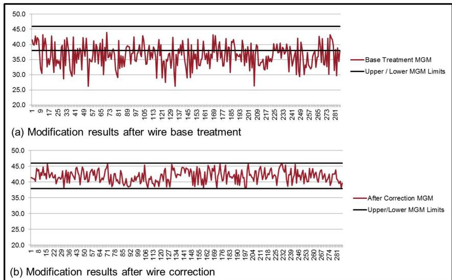
Figure 6: Series production results for Modification after the base treatment and correction of 281 ladles show the need for a two-step casting process to simultaneously eliminate flake graphite and shrinkage defects in complex CGI components.
