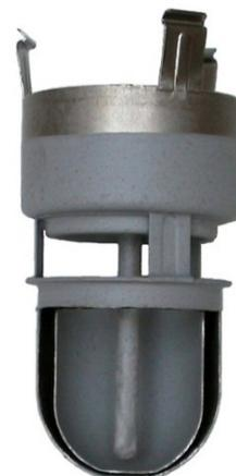
(b) SinterCast immersion sampling steel cup with regulated heat loss, showing the protective tube for the containment of the reusable thermocouples.
