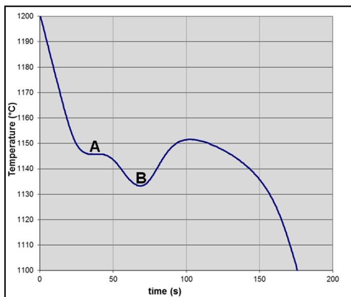
Figure 2: In hypereutectic irons, the heat released by primary austenite results in a thermal plateau at Point A. Thereafter, the onset of the eutectic solidification of graphite and austenite defines the undercooling at Point B, and the graphite growth beyond.
