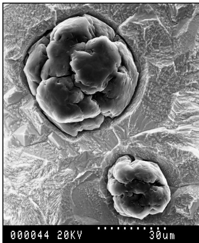
*Figure 3: A typical 50 µm graphite nodule contains more than 10<sup>20</sup> carbon atoms. The rate of consumption of carbon from the liquid, determined by the shape of the graphite, controls the heat released during solidification and provides the opportunity for measurement and control.*
