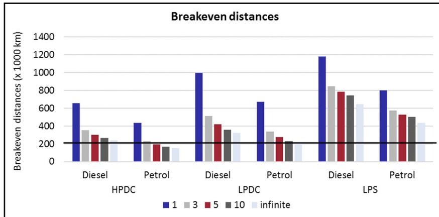
Figure 5: Effect of the number of recycling loops on the energy breakeven distance. The horizontal line represents the global average vehicle life of 210,000 km
