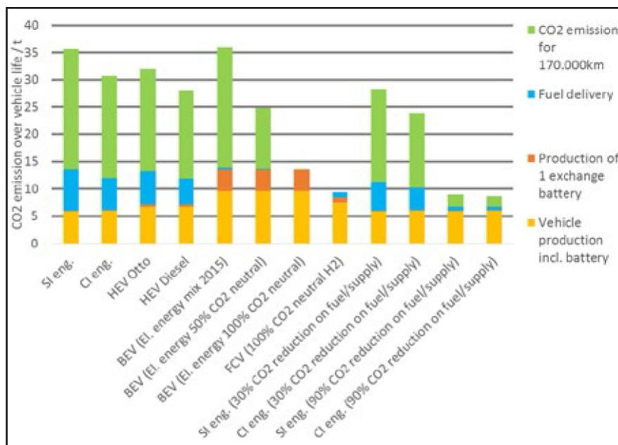
Figure 7: Life cycle analysis conducted by FEV GmbH, Germany, based on a 170,000 km vehicle lifespan [5]
