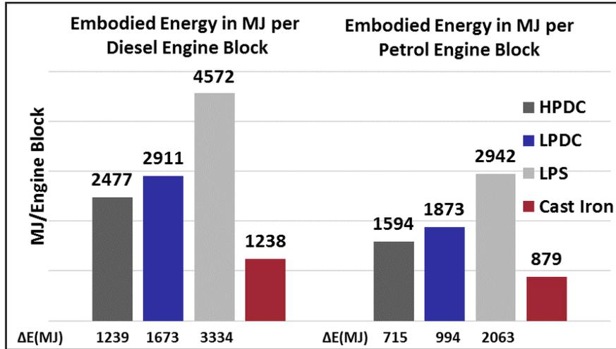
Figure 4: Embodied energy for diesel and gasoline engine cylinder blocks, and the energy differentials relative to cast iron
