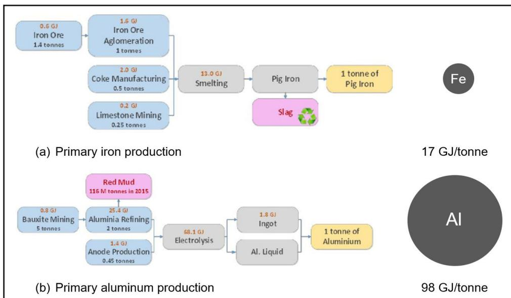
Figure 1: Process steps and associated energy to produce one tonne of primary metal
