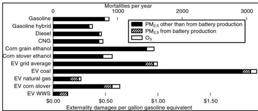
Figure 8: The generation of electricity from fossil fuels emits CO<sub>2</sub>, NO<sub>x</sub>, particulates and toxins. Life cycle studies show that a conversion to electric vehicles will not necessarily result in an improvement of public health [7]
