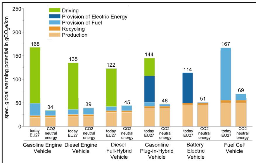
Figure 6: Life cycle analysis conducted by IAV GmbH, Germany, based on a 200,000 km vehicle lifespan [4]
