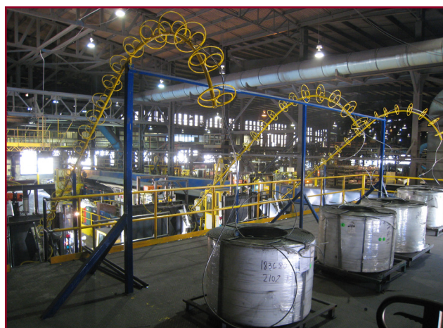
Figure 2: Multiple wirefeeders for base treatment and correction
