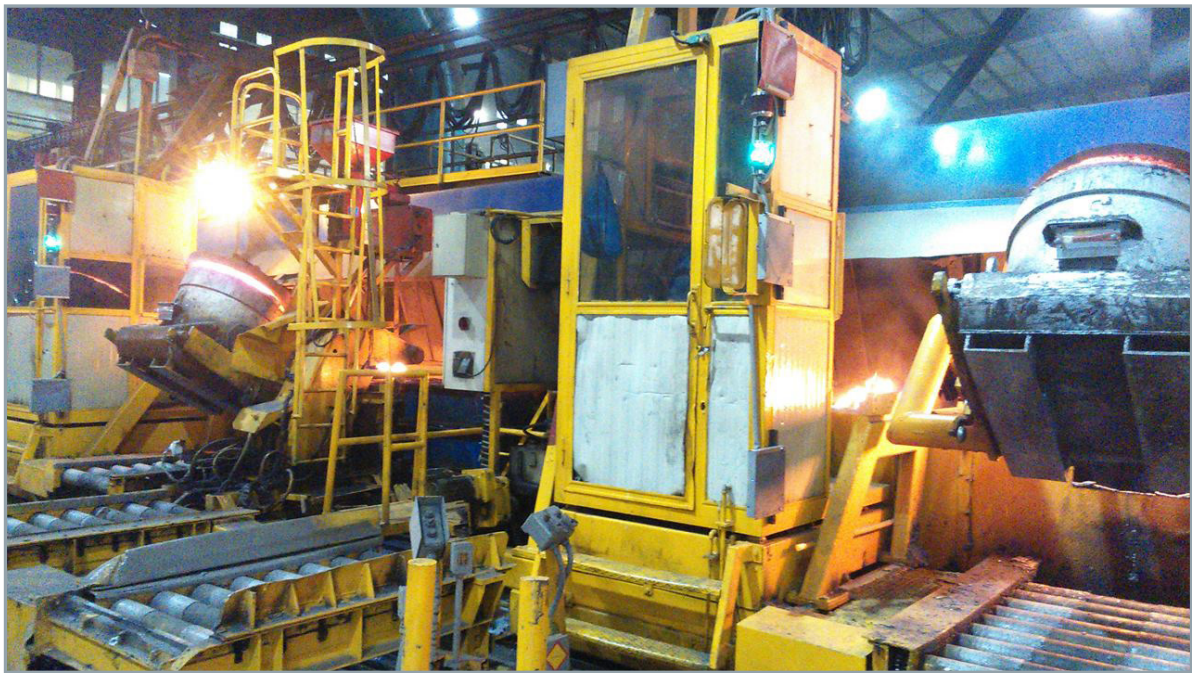
Figure 3: System 3000 Plus : parallel pouring of SinterCast-CGI cylinder blocks
