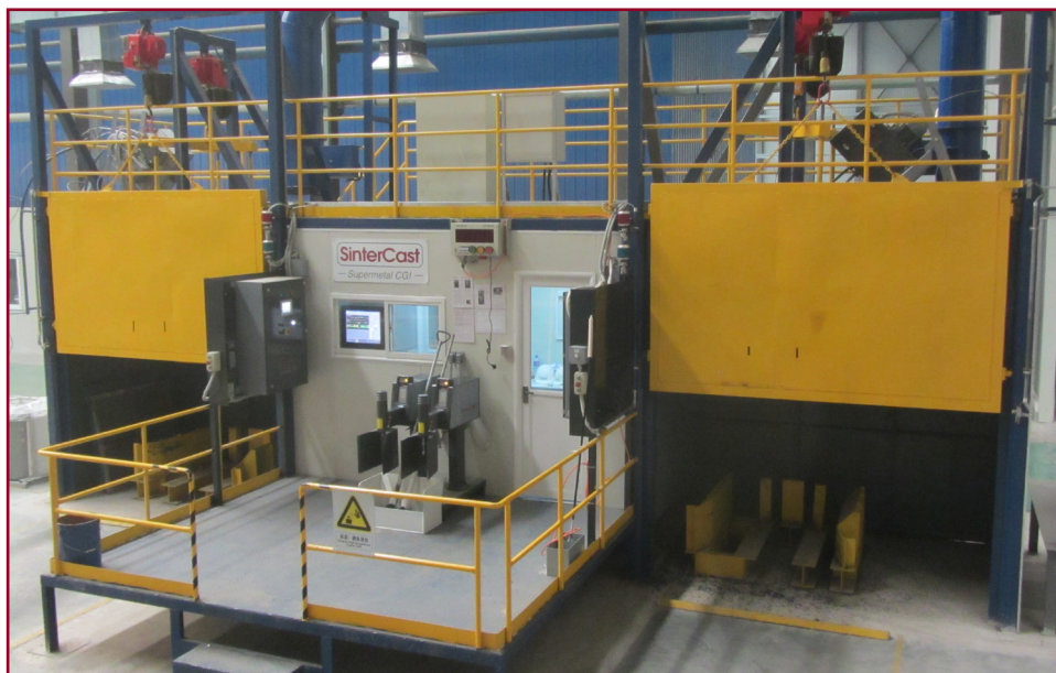
Figure 1: System 3000 Plus base treatment and correction stations
