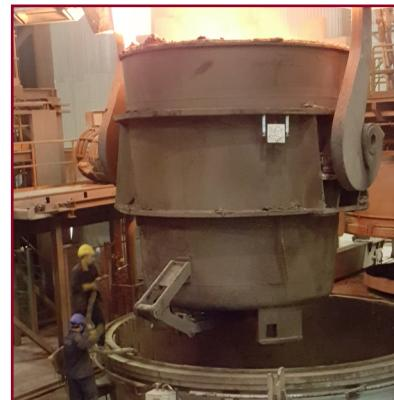
*RFID tags or 2D optical matrix plates (shown) can be used to identify ladles.*
