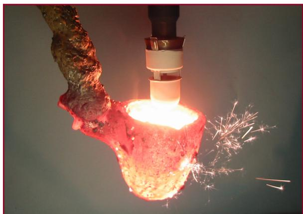
SinterCast Immersion Sampling
