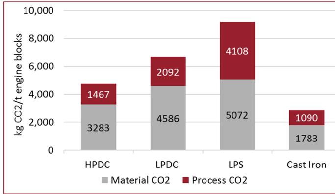
Figure 6: Summary of CO<sub>2</sub> burden per tonne of good castings for the different casting processes
