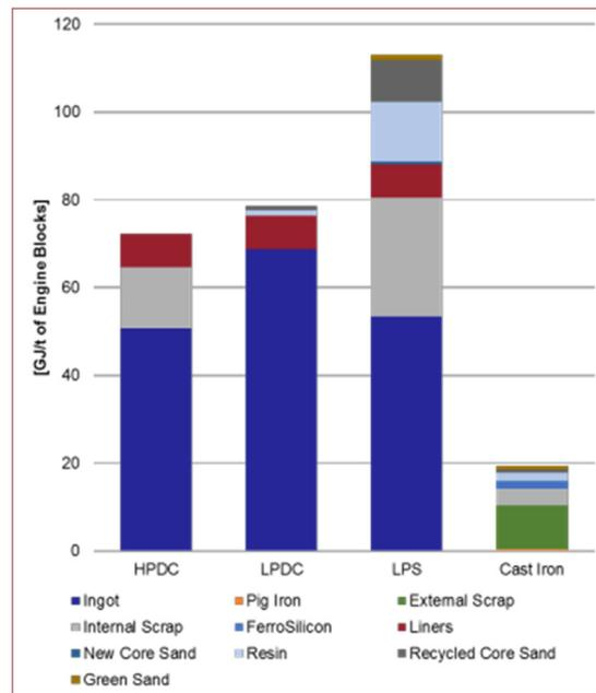
Figure 2: Breakdown of the embodied material energy (GJ) per tonne of cylinder blocks
