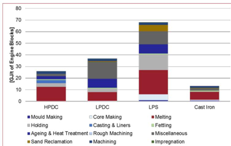
Figure 3: Breakdown of the embodied material energy (GJ) per tonne of cylinder blocks
