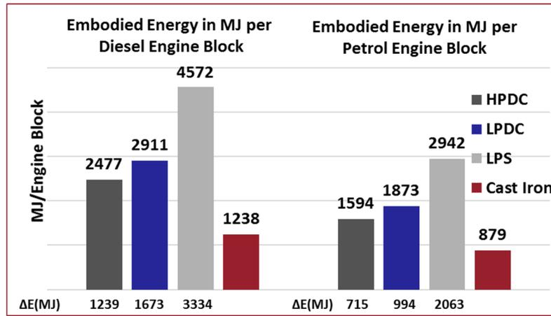
Figure 4: Embodied energy for diesel and petrol engine cylinder blocks, and the energy differentials relative to cast iron
