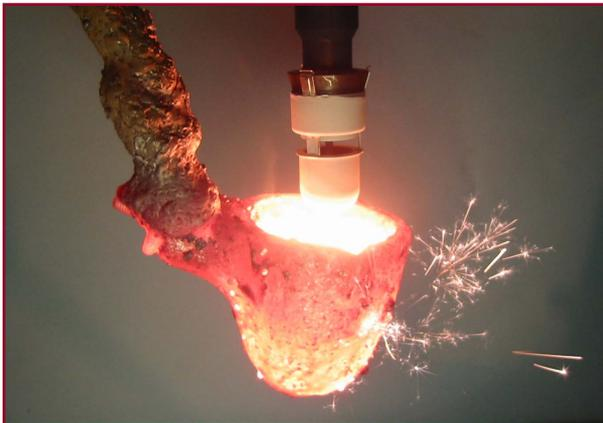
Figure 2: SinterCast Immersion Sampling
