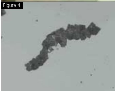
Top to bottom: Figure 1: Daros Piston Rings facilities at Molnlycke near Gothenburg; Figure 2: Graphite shape in Darcast manufactured by the Foot Mineral method; Figure 3: SinterCast control system at Daros Piston Rings foundry; Figure 4: Graphite shape in Darcast manufactured by the SinterCast method.
