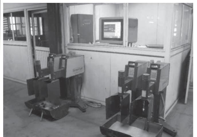
Figure 5: SinterCast System 3000 Plus – SAMs and OCM.
