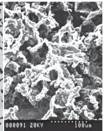
Figure 2: Deep-etch SEM photo of CGI microstructure.
