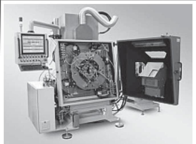
The latest **LamaCaster H65 Mk3** die casting machine assures quality and consistency of precision zinc die castings up to 60 grams where the highest levels of surface finish and minimum porosity are required. Many major upgrades have been made to the Mk3 machine to improve the overall machine capability.
