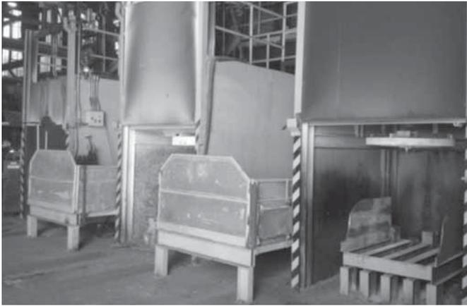
Figure 9: System 3000 *Plus* – base treatment (center) and correction enclosures (north and south).
