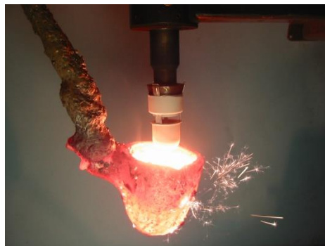
The patented SinterCast Sampling Cup is the only thermal analysis device in the world that uses a high accuracy steel vessel and reusable thermocouples
